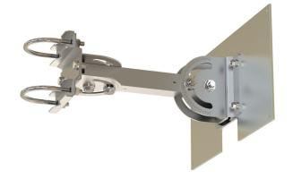
The AccelTex Solutions articulating mount for the Cisco AIR-ANT2566P4W-R allows installers to articulate the antenna horizontally and vertically to cover a specified area. This heavy duty mount is suitable for a wall, ceiling or pole installation and with the inscribed degree markings, provides maximum and precise articulation for the antenna.
